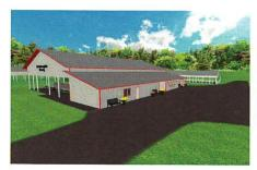
Pole frame construction 120' x 72' building with a 120' x 24' lean-to.
